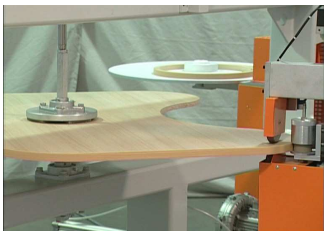
First phase: clamp of the panel, glue of the edge and start edge banding
