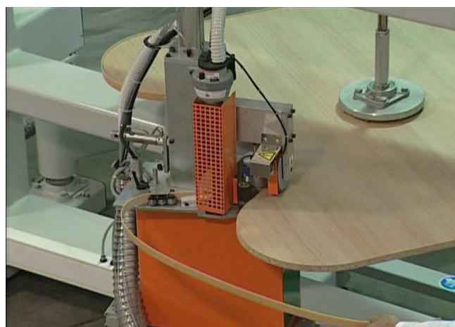
First phase: clamp of the panel, glue of the edge and start edge banding
