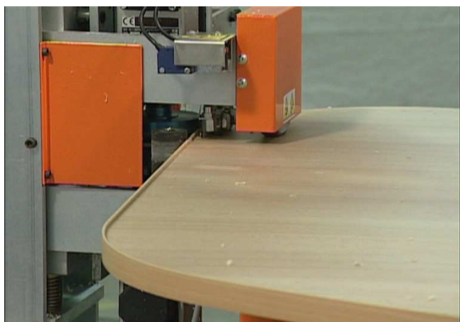
Second phase: Trimming of the edge
