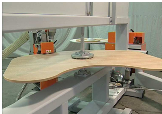
Second phase: Trimming of the edge
